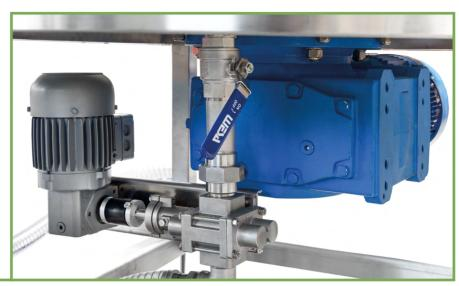
Emergency drainage tap at the bottom of the fermenter for easy emptying of dough or cleaning water
