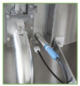
Integrated pH sensor to measure automatically the acidity level for sourdough or pre-ferment
