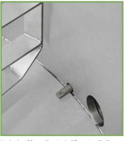
Interior view of the new Hematronic pH fermenter with pH sensor and adapted agitator
